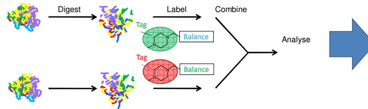
Figure 1: The analysis pathway for the saliva samples. Protein samples are digested, labelled with iTRAQ 115 and 118, combined and analysed with 2D LC-MS/MS
