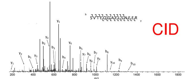
Figure 2: The collision induced dissociation (CID) mass spectrum of the triply charged peptide ion [iTRAQ-SVTEQGAELSNEER]<sup>3+</sup>. Complete coverage is observed.
